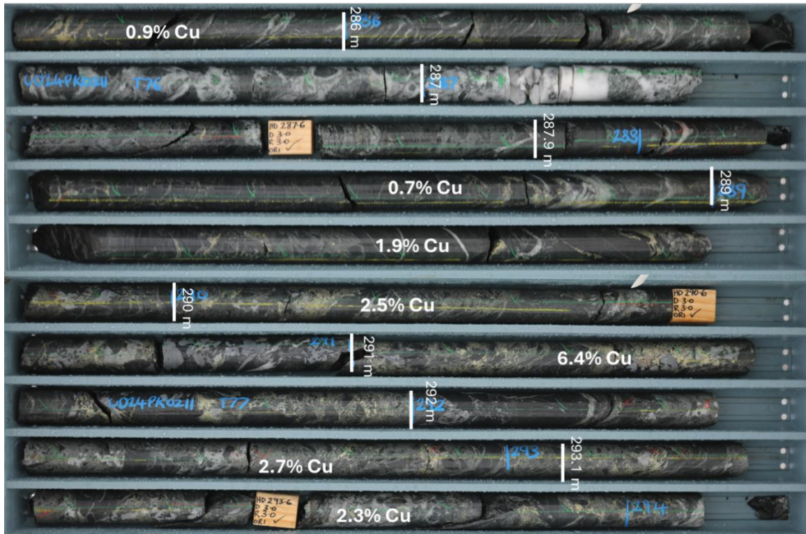
Figure 5: A section of Kairos Deeps drillhole UD24PK0211 highlighting 6.4m at 2.7% copper from 287.9m.
