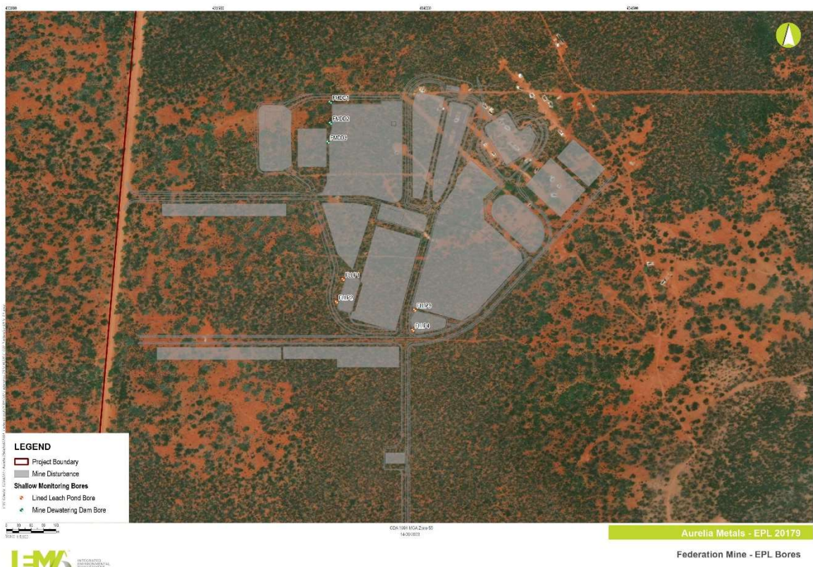
Figure 6 – Federation Groundwater Monitoring bores
