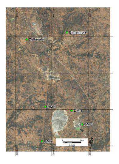
Figure 2: Location of dust gauges on PGM Mining Leases.
