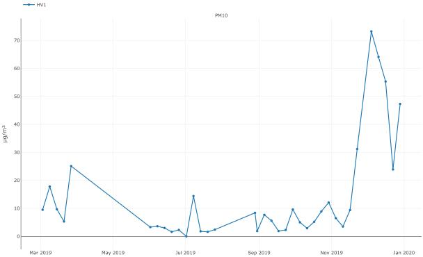
Dargues mine has one High Volume Air Sampler (HVAS). The unit is designed to sample Particulate matter less than  $10\mu m$  (PM10). The monitoring samples are sent to Australian Laboratory Services monthly for analysis.
