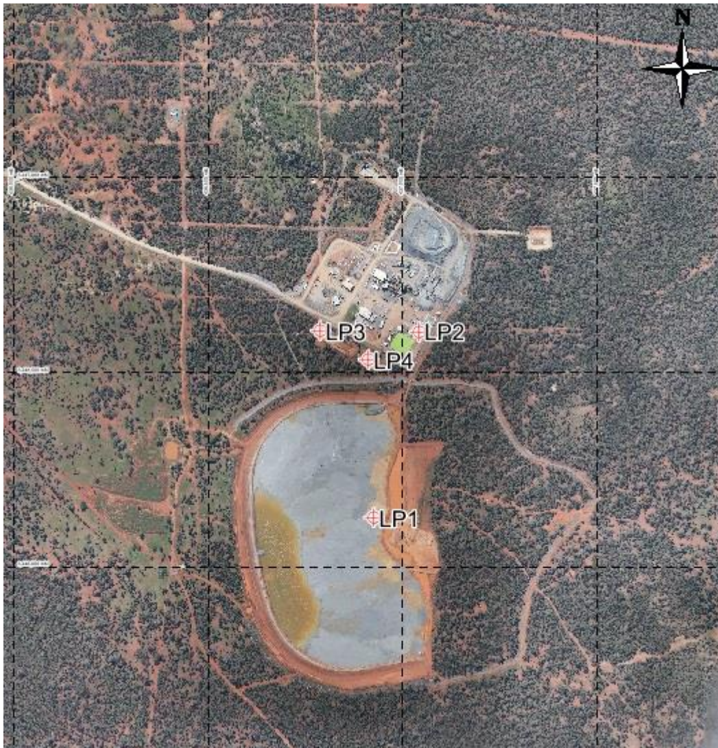
Figure 3. Licensed surface water monitoring points located onsite.
