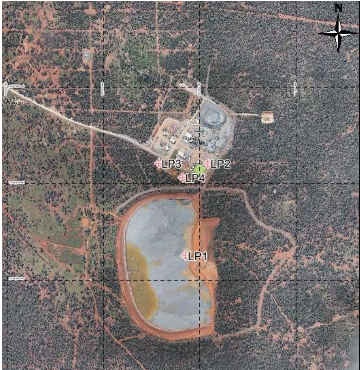
Figure 3. Licensed surface water monitoring points located onsite.
